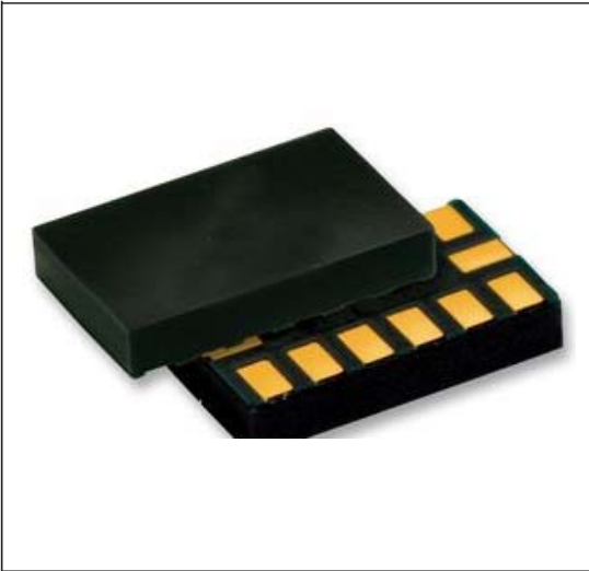
LGA14 (3x5x0.92mm) Pitch 0.8mm Land Grid Array Package
